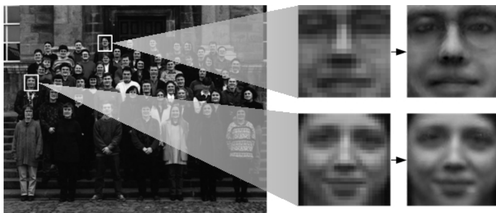
Figure 4: Super resolution and face detection. All the faces in the group photograph were detected. Two of them have been enlarged to show the original image and the enhancements using super resolution [11].
