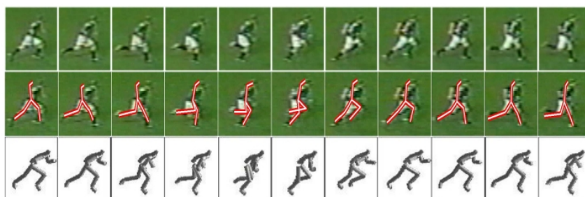
Figure 5: Action recognition at a distance. The first row shows a zoomed in shot of the footballer, which is clearly represented at really low resolution. The second row shows the 2D skeleton of the footballer taken by taking motion from the images in the top row and learned models of where the joints in the person are likely to be. The third row shows the 3D skeletonisation of the footballer by taking motion information extracted from the first row and the 2D skeletons of the second row.
