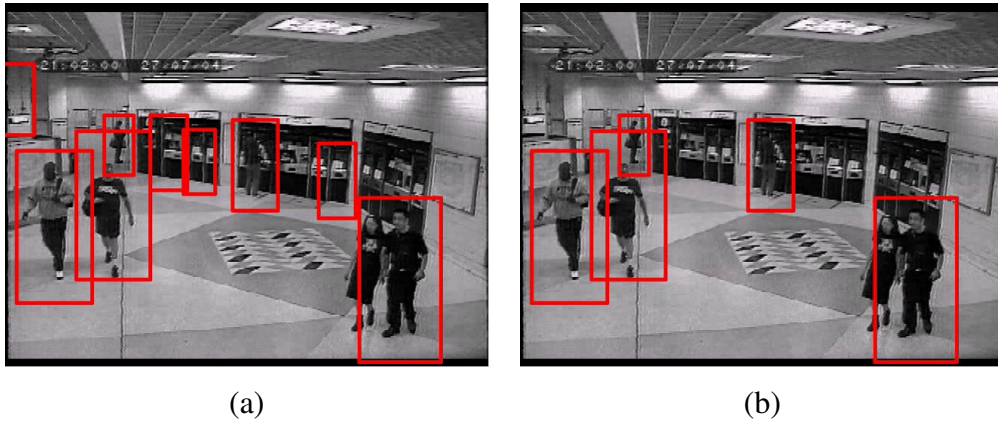
Figure 3: Results reproduced from [22] of the person detection system in a busy tube station. The images show the results without using the motion information to detect the people (a) and the system when just using person detector, using the motion information(b).
