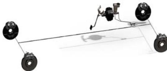
Figure 1: A typical disc brake system, from [1].
