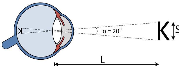
Figure 8: Angle  $\alpha = 60 \text{ minutes} * \text{arc tan}(S/L)$ .
