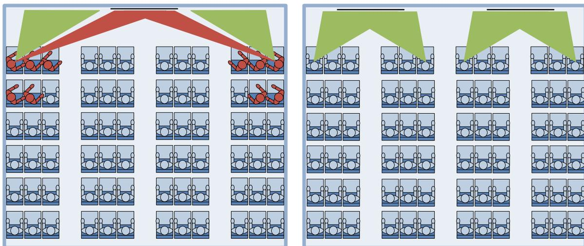
Figure 6: Horizontal viewing angles with a) one centrally positioned projection screen and b) two projection screens.
