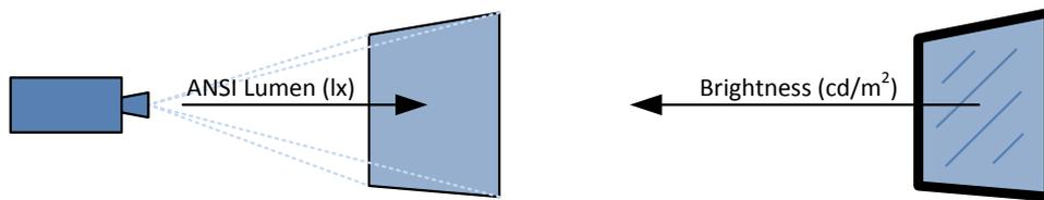
Figure 12: Projection screen with receiving light in lx and LED display with radiating light in  $\text{cd}/\text{m}^2$ .
