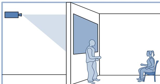
When back view projection is possible, for example when there is space behind the projection screen, then this is most advisable. With back view projection the lecturer is never in the light beam, hence projection is not interrupted. Moreover, the annoying sound of the cooling fan has disappeared to the space behind the projection screen.
