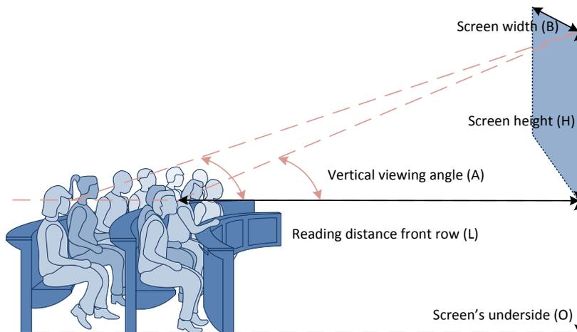
Figure 1: Positioning a presentation screen in the lecture hall; important dimensions are screen's underside (O), vertical viewing angle (A), reading distance from front row (L), height of presentation screen (H) and width of presentation screen (B).
