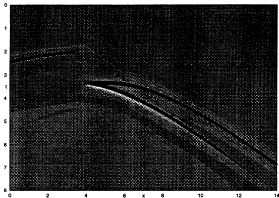
Fig. 2c. Ray-tracing result for a smooth model with H = 0.1 compared to a finite-difference solution with H = 0 .
