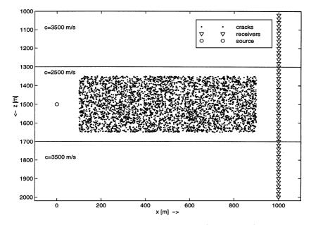
FIG. 5. Geometry of the crosswell simulation. A low-velocity layer (c = 2500 m/s), containing 4000 randomly positioned cracks, is embedded in two high-velocity layers (c = 3500 m/s). The seismic source is located in the low-velocity layer (on the left side), whereas the receivers are positioned in a vertical borehole on the right.
