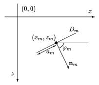
FIG. 1. Each crack is represented by a line segment  $D_m$ . It can be characterized by the position of its center,  $\mathbf{x}_m = (x_m, z_m)$ , its half-width  $a_m$ , and the angle  $\varphi_m$  with the horizontal. The z-coordinate indicates depth; the x-coordinate refers to the horizontal position. The unit vector normal to the crack is defined as  $\mathbf{n}_m = (\cos \varphi_m, \sin \varphi_m)$ .
