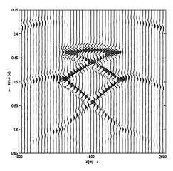
FIG. 6. Wave field transmitted through a low-velocity layer containing 4000 randomly oriented cracks. The geometry is shown in Figure 5. The wave field is clearly "trapped" in the layer.
