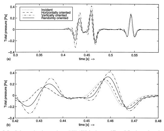
FIG. 7. Detailed comparison for a receiver at (1000, 1500) for the case of Figure 5. Results are shown for the following cases: (1) no cracks (incident field only), (2) all cracks horizontally aligned, (3) all cracks vertically aligned, and (4) cracks randomly oriented. (a) Results between 0.3 and 0.6 s, (b) detail between 0.42 and 0.48 s.
