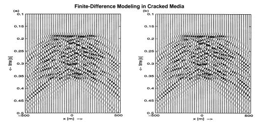
FIG. 3. Comparison of the scattered fields of the FD method (a) and BIE method (b). An incident plane wave is scattered from a region with 3000 horizontally oriented cracks, embedded in a homogeneous medium with sound speed c = 2500 m/s. The scattered wave field is shown at z = 0 m.
