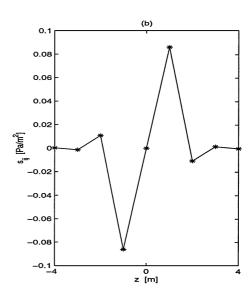
Fig. 2. Numerically constructed source distribution of a horizontally oriented crack as a function of x and z (a) and a vertical cross-section through the center of the crack (b). The source values are computed by applying the discrete wave operator to the numerically computed values of the scattered pressure in the grid points.
