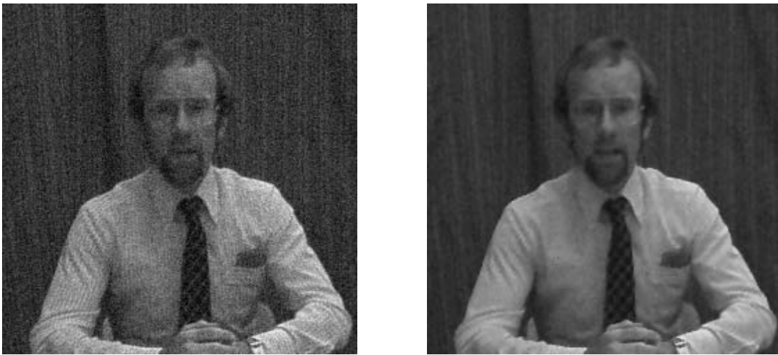
FIGURE 5.10: THE OBSERVED “TREVOR” SEQUENCE AT 10DB SNR AND THE RESULT AFTER APPLYING THE LLMMSE FILTER SUPPORTED BY THE RANGE TEST
