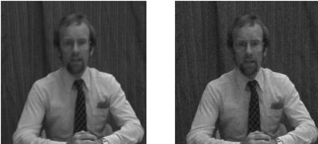
FIGURE 4.9: FILTERED FRAMES WITH THE PROPOSED DECOMPOSITION METHOD WITHOUT (LEFT) AND WITH (RIGHT) MOTION COMPENSATION FOR AN SNR OF 10dB
