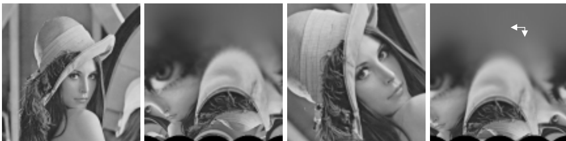
(a) Original image (b) LPM of (a) (c) Scaled, rotated (d) LPM of (c)
