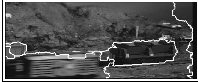
Figure 4.15: Object edges superimposed on the 10th frame of the “train” sequence with forward motion estimation and labeling ( \{d_s = 1, s \in [1 \dots K]\} ). The absence of a correct match in the next frame causes misclassifications in occluded areas.
