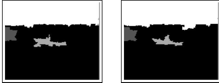
Figure 4.8: Label field used for the 9th frame of “coast guard” sequence and label field obtained for the 10th frame using spatial and temporal constraints
