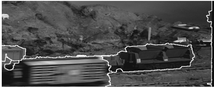
Figure 3.22: Object edges derived from the label field of fig. 3.21(b) superimposed on the original frame
