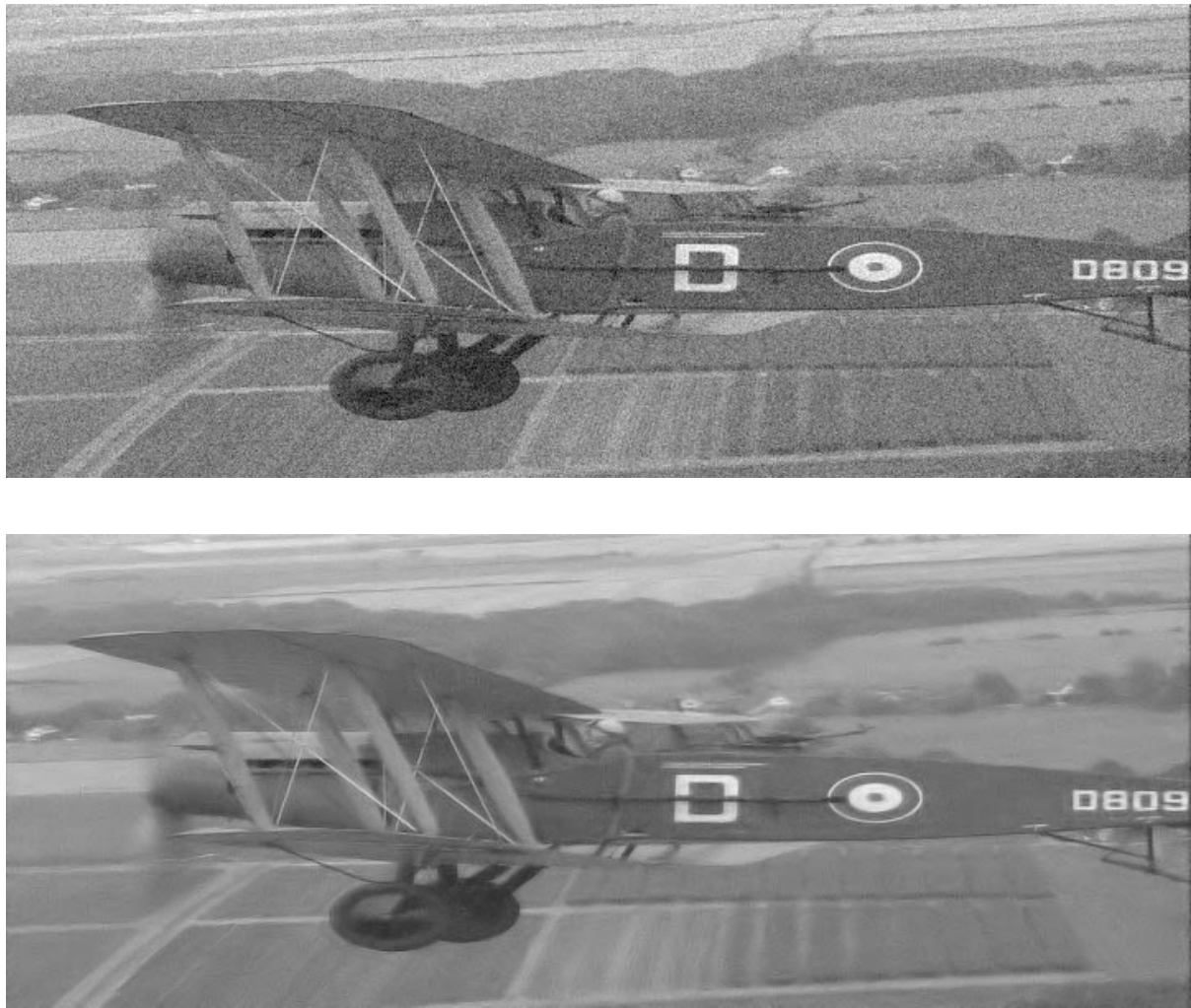
Figure 5.8 Top: noisy field from Plane sequence with noise variance 225 (PSNR = 23.5 dB). Bottom: filtered result from the 3D pyramid filter. (Sequence available by courtesy of the BBC).
