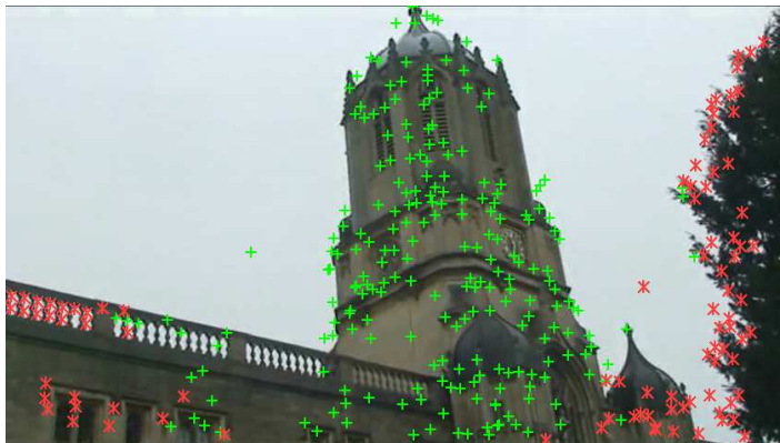
Figure 6.8: The examples of “good” feature points. The green points are good points and the red ones are those being filtered out.
