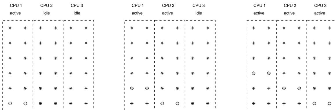
Figure 29: The first stages of the staircase parallel solution of the lower triangular system  $Lx = b$ . The symbols denote the following: \* nodes to be calculated, o nodes being calculated, and + nodes that have been calculated.
