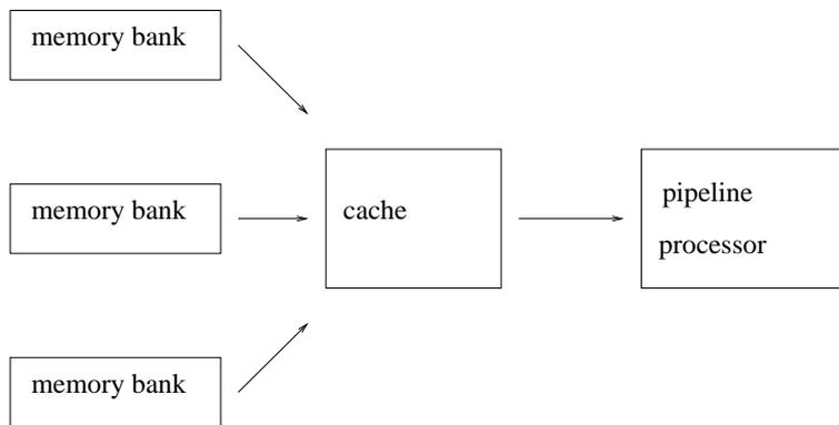
Figure 18: A pipelined processor with memory interleaving and cache
