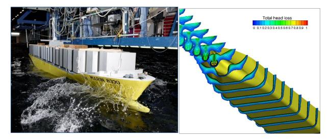
**Project Background** Reducing fuel consumption of a ship can be done by improving the hull form design and/or by increasing the efficiency of its propeller. Computational Fluid Dynamics (CFD) plays an ever-increasing role to achieve this, as it permits extensive design studies prior to any model testing. Instead of using one CFD-computation, automatic optimization procedures can be used to evaluate a series of hull forms and propellers.
