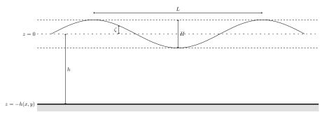
h(x,y) Water depth H Wave height  $\label{eq:logistical} \begin{array}{l} L \mbox{ Wave length} \\ \zeta(x,y,t) \mbox{ Elevation of the free surface} \end{array}$
