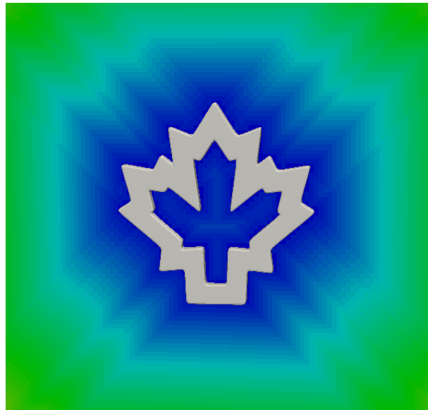
Figure 9: Artificial signed distance function of a maple leaf (Computed using our approach)
