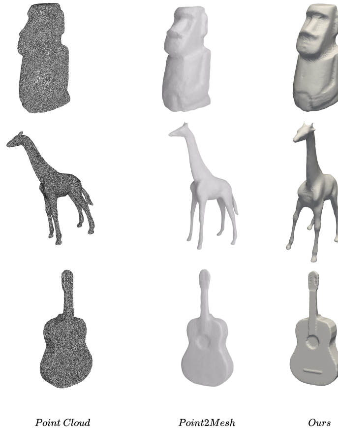
Figure 25: Few point cloud geometries from Point2Mesh [21] along with its output. It can be noticed that our wrap algorithm produces equally smooth results except for a few artefacts created as a result of morphological operators.
