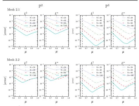
Fig. 2 The  $L^2$  and  $L^\infty$  errors in log scale of the filtered solutions with various scaling  $H=h^\mu$ ,  $\mu\in[0.6,1.0]$ . The black dashed line marks the location of  $\mu_0=\frac{2k+1}{3k+2}$ . The DG approximation is for the linear equation (5.1) with polynomials of degree k=2,3 for Meshs 2.1 and 2.2
