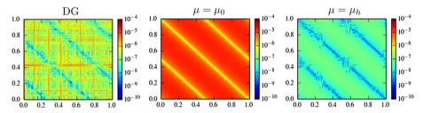
**Fig. 8** Comparison of the pointwise errors in log scale of the DG approximation together with two filtered solutions (using scaling order  $\mu = \mu_0$  and  $\mu = \mu_h$ ) for two-dimensional linear equation (5.3) for Mesh 2.2 (2D.  $\mathbb{P}^2$  and  $N = 160 \times 160$ )
