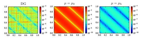
**Fig. 7** Comparison of the pointwise errors in log scale of the DG approximation together with two filtered solutions (using scaling order  $\mu = \mu_0$  and  $\mu = \mu_h$ ) for two-dimensional linear equation (5.3) for Mesh 2.1 (2D,  $\mathbb{P}^2$  and  $N = 160 \times 160$ )
