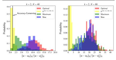
**Fig. 4** The comparison for the performance of different scalings: optimal scaling, theoretical scaling, maximum scaling, the new scaling for k=2. The x-axis is the value of  $\|u-u_h\|_0/\|u-u_h^*\|_0$ , clearly, the larger the value, the better the filtering. In addition, we mark the accuracy-conserving position x=1 with a black line
