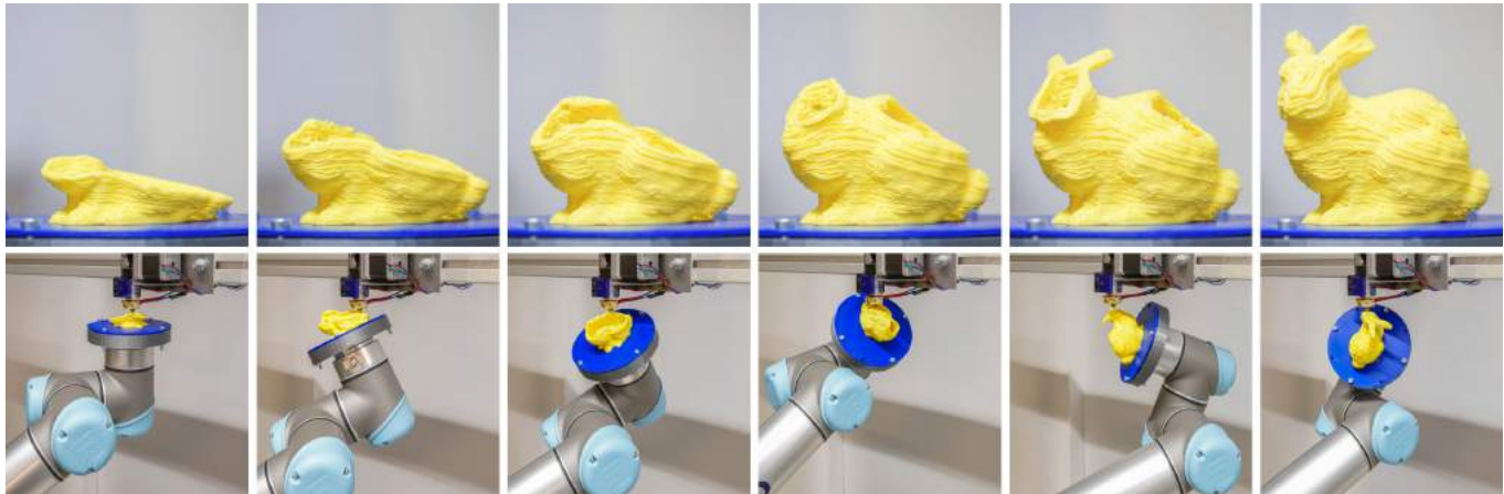
Fig. 1. Our method enables support-free 3D printing of solid models. By exploiting all 6 degrees of freedom (translations, rotations) and depositing material along curved layers, we make support structures unnecessary in most cases. This increases further the flexibility offered by 3D printing, such as freeing designers from support constraints on complex parts.
