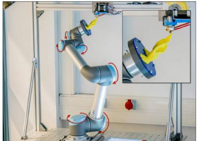
Fig. 2. The hardware of our multi-axis 3D printing system using a 6DOF robotic arm, where each red arrow indicates a motor to provide one rotational DOF. The printer head is fixed in our system so that the orientation change for material accumulation is realized by moving the end effect of the robot arm inversely.
