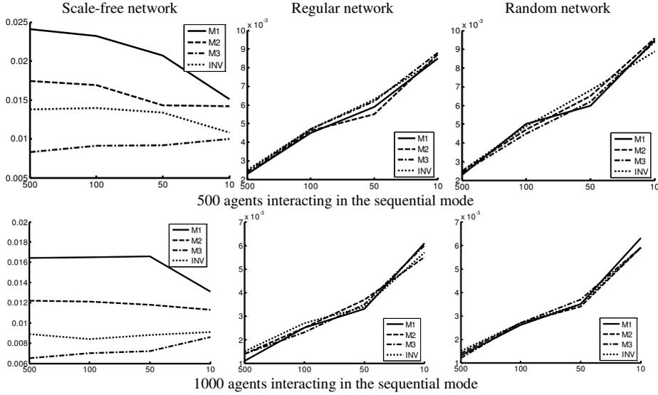
**Fig. 8.** Mean RMSE errors for the proposed abstraction methods  $M1$ - $M3$  and the invariant-based method ( $INV$ ) in the sequential mode; the horizontal axis is the average time between messages.
