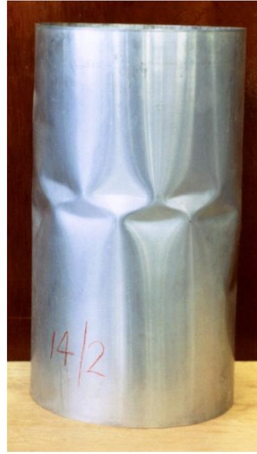
Figure 4. Yoshimura buckling of an aluminium cylinder
