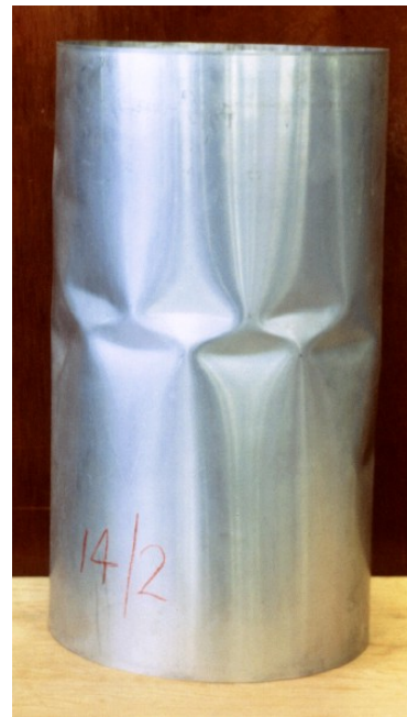
Figure 4. Yoshimura buckling of an aluminium cylinder
