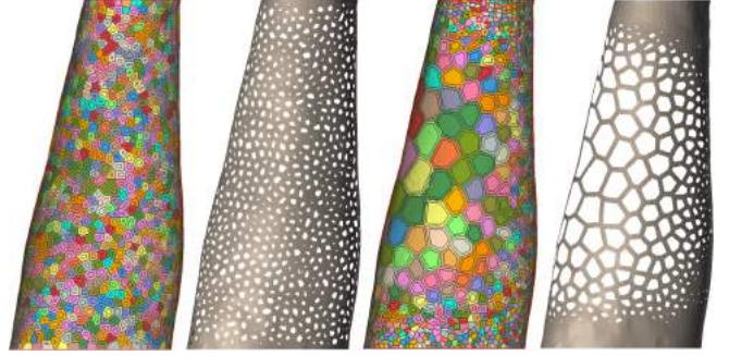
Figure 6. Some regions will be completely covered if the cell-removal mechanism is not included in our algorithm. (Left) a cast with uniform distribution of 500 cells, and (right) a cast with the same number of cells but having adaptive distribution. As a result, discomfort at fully covered regions (although having low thermal-comfort sensitivity) will dominate the overall perception of comfort.
