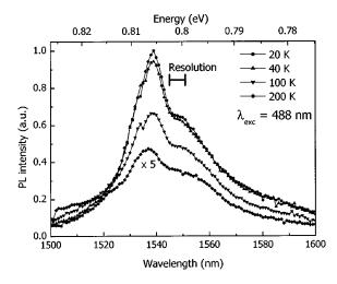
FIG. 2. PL spectra of an Er-implanted silicon-infiltrated colloidal crystal after annealing at 400 °C. Spectra are taken at different temperatures. The broad spectrum and the PL quenching with increasing temperature are characteristic features for Er in a-Si. Pump wavelength is 488 nm.
