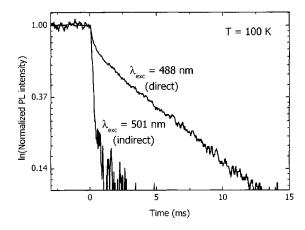
FIG. 5. Normalized PL decay measurements, taken at 1.536  $\mu$ m and 100 K (see Fig. 3) for two different excitation wavelengths. After excitation at 488 nm the laser is switched of at t=0 and the decay curve shows a slow decay contribution from  $\text{Er}^{3+}$  in silica, together with a fast decay from  $\text{Er}^{3+}$  in Si. Using indirect excitation (501 nm) only  $\text{Er}^{3+}$  in Si is excited and the corresponding fast decay component is observed.
