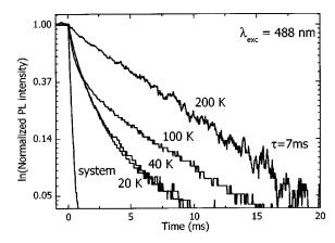
FIG. 4. Normalized PL decay measurements, taken at 1.536  $\mu$ m at different temperatures (see for spectra Fig. 3). After excitation at 488 nm the laser is switched of at t=0. The PL decay measurements at 20 and 40 K are composed of PL from  $Er^{3+}$  in Si (fast decay) and  $Er^{3+}$  in silica (slow decay). For higher temperatures the PL of  $Er^{3+}$  in Si quenches and the contribution from  $Er^{3+}$  in silica remains.
