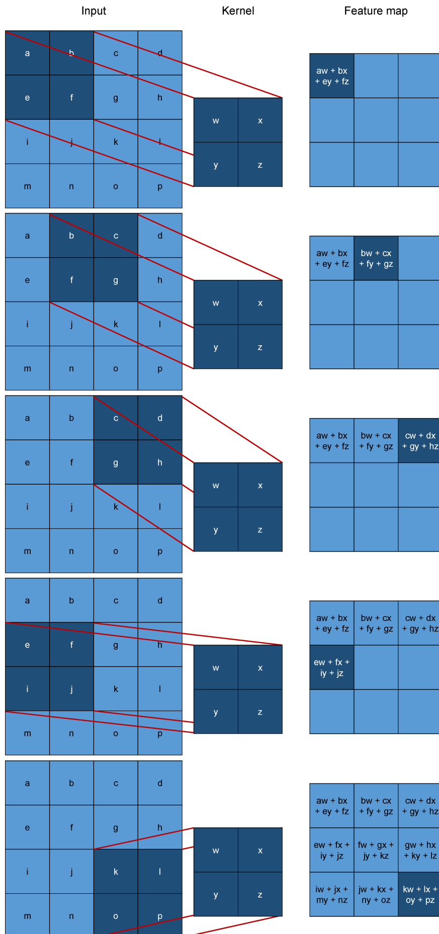
Figure 3.3: A kernel of 2 \times 2 slides over the input feature map of 4 \times 4 . At each position it calculates the sum of the multiplications of each kernel entry with their corresponding overlapping window entry. The result of the calculation is positioned in the output feature map at the same location. The kernel slides with one stride (stepsize) to the right and below. Only the first four and the last windows and their calculations are given in this figure [13, 17].
