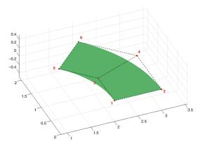
• the shape of  $\Omega_h$  is fully specified by the set of **control points**  $\mathbf{x}_i \in \mathbb{R}^d$
