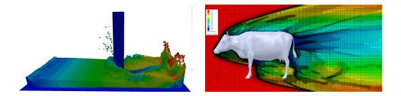
Left: wave-structure interaction, LS-DYNA; right: supersonic flow around a cow, Siemens FloEFD
