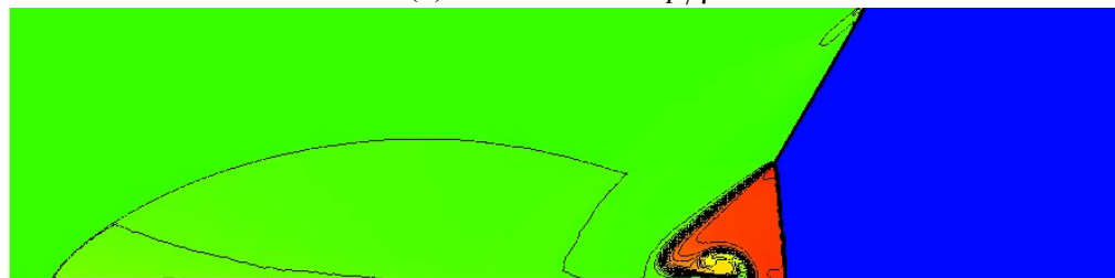
Fig. 5.21. Double Mach reflection at t = 0.2 : FEM-TVD scheme (50 contours).
