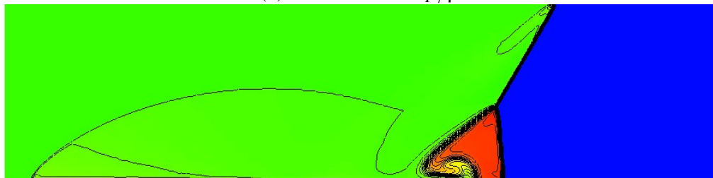
Fig. 5.19. Double Mach reflection at t = 0.2 : FEM-TVD scheme (50 contours).
