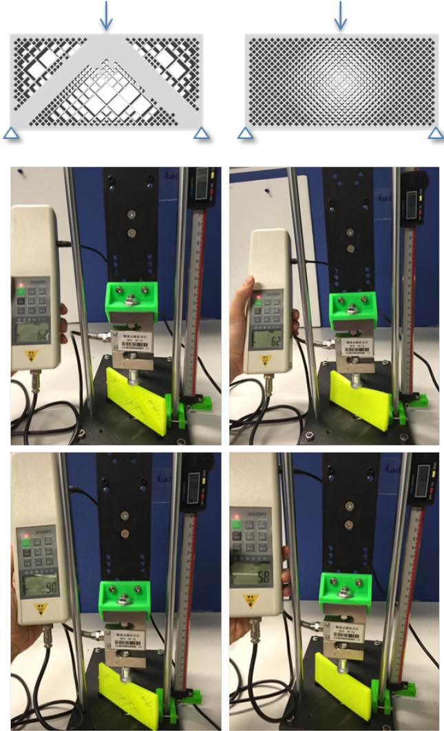
Figure 12: First row: The adaptively refined infill (left) and the uniform infill (right) consume the same amount of material. Second row: Under the same applied force of  $62\text{ N}$ , the optimized infill deforms by  $2.11\text{ mm}$ , while the uniform one has a larger deformation of  $4.08\text{ mm}$ . Third row: When both deform by  $3\text{ mm}$ , the optimized infill supports a force of  $90\text{ N}$ , while the uniform one supports a smaller force of  $58\text{ N}$ .
